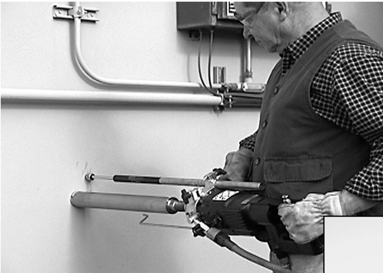
A drilling aid is included to assist in starting freehand drilling without walk. Once the drill bit is started, the drilling aid can be moved out of the way.
